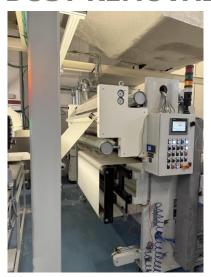
Xstream high speed non contact surface cleaning technology with iONstream AUTODC ionisation system
